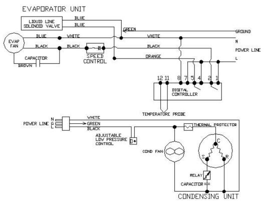
Fig. 2.5 VINO6500SSR Electrical Wiring Diagram (DIGITAL CONTROLLER)
